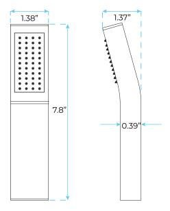
The minimum required water pressure is 0.05 MPa (0.5 bar).
